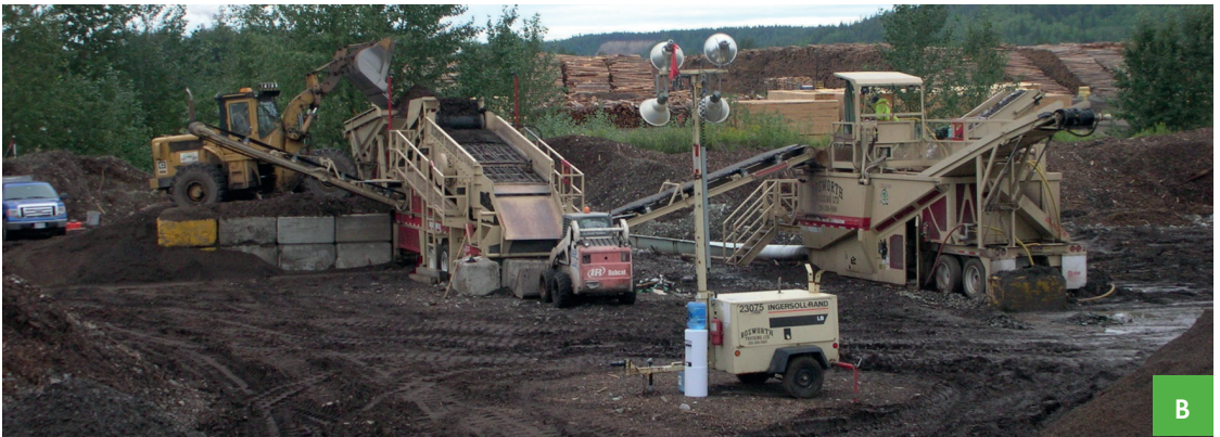
Figure 2. Biomass preparation through screening (A) and washing (B).
