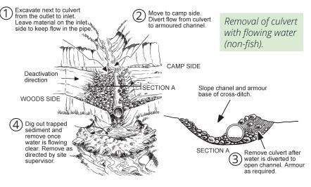
increase the need for sediment control. Improved sediment control can be achieved by temporarily diverting flow to dewater the site before construction starts. In all cases, install sediment control downstream prior to the start of any earthworks at the site.
