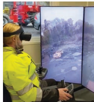
Virtual reality-based teleoperation of forwarder (Courtesy of Skogforsk's Troedsson Forestry Teleoperation Lab)
