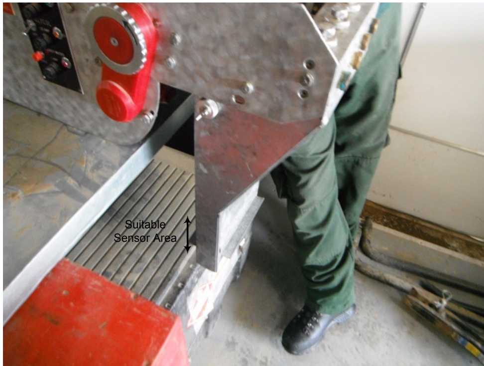
Figure 4. Possible sensor location on the PSD unit.
