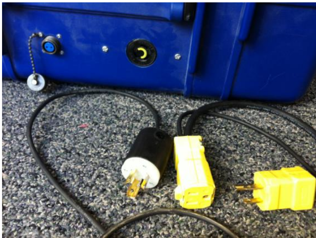
Figure 6. Alberta helitorch interface cable and connection to existing logging unit.
