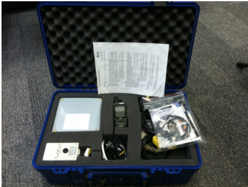
Figure 1. Current ESRD aerial helitorch logging unit.
