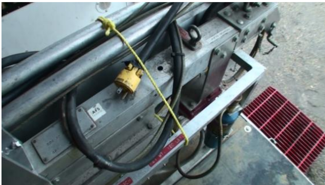
Figure 5. Power connection on the Alberta helitorch.
