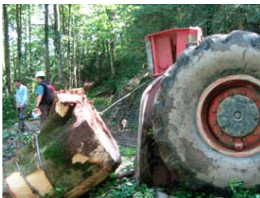
Figure 1. 19-mm Amsteel Blue used to extract a 5.2 m 3 beech stem 80 metres up-slope (70%).
