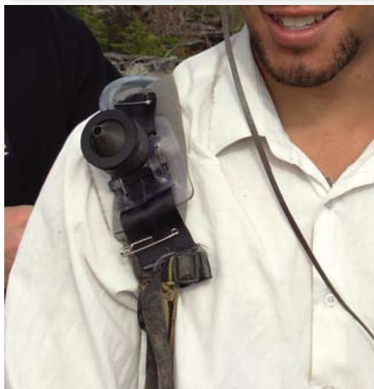
Figure 2. Nozzle for sampling dust inhalation by planter.
