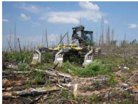
Figure 1. ( left ) The Bräcke M36a moulder mounted on an eight-wheeled Timberjack 1710D forwarder.
