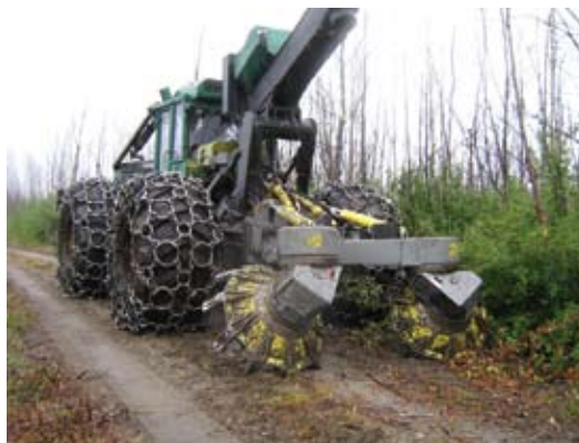
Figure 3. The Bräcke T26a powered disc trencher mounted on a John Deere 748G skidder.
