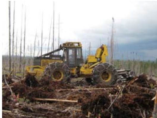
Figure 4. The TTS-Delta powered disc trencher mounted on a John Deere 748E skidder.
