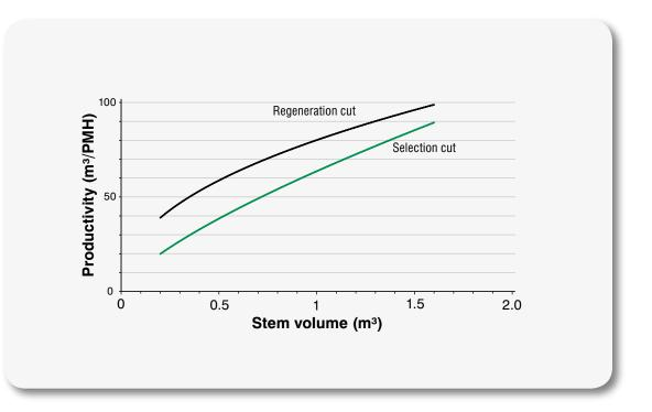
Figure 3. Regression equations for the productivity of the feller-bunchers in the selection cut (Productivity =  $63.628 \times \text{Vol.}^{0.7227}$ ,  $R^2 = 0.90$ ) and the regeneration cut (Productivity =  $80.097 \times \text{Vol.}^{0.4471}$ ,  $R^2 = 0.97$ )
