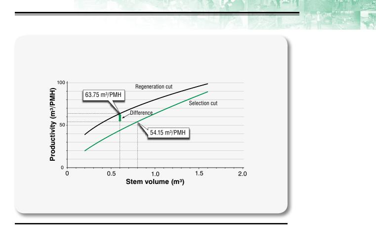
Figure 4. Example of a productivity comparison between the two treatments in a given stand. The cost difference (green arrow) accounts for the differences in the mean harvested stem volume that result from the different treatment prescriptions.
