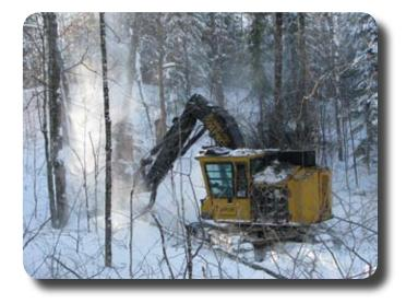
Figure 2. A fellerbuncher working in a selection cut.
