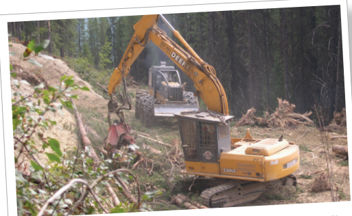
Harvesting of the right-of-way timber was fully mechanized; here a skidder and processor are working at a landing.
