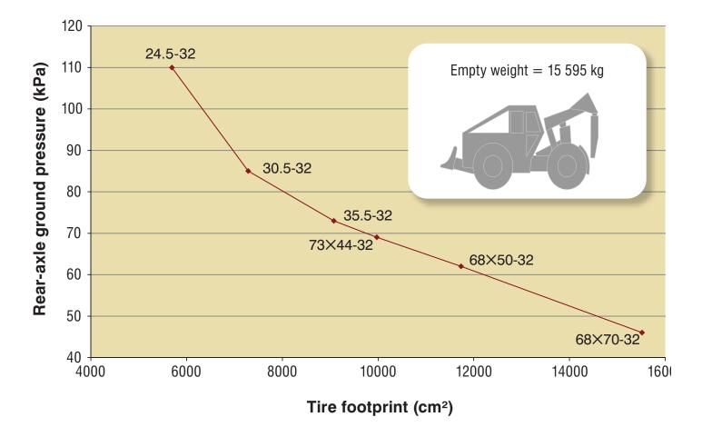
which the load is distributed. This can be particularly valuable for the rear axle of fully loaded forwarders. For forwarders working in commercial thinning or other partial cutting applications, it may be difficult to use wide tires because of the narrow spaces between trees, so the use of tracks is an important way to reduce ground pressure. Adding tracks to a bogie axle can reduce the ground pressure by approximately 50%, as Figure 4 shows using the example of a 14-tonne forwarder.
