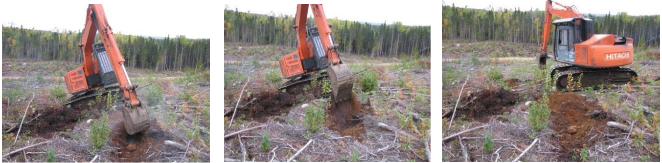
Figure 2. View of mounding sequence with excavator.
