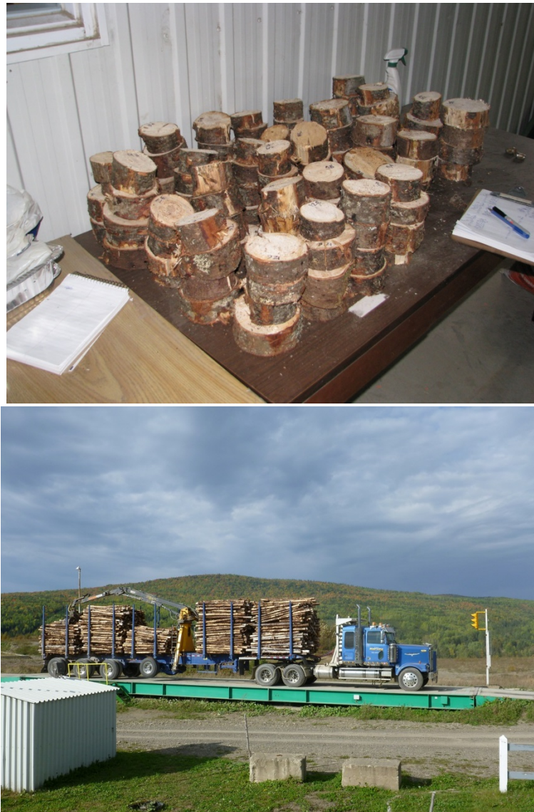
Figure 3. Disc samples (top) and pile weighing (bottom) to determine moisture content.
