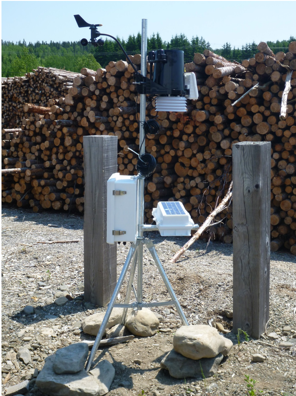
Figure 5. Davis Vantage Pro2 Plus weather station used to measure on-site precipitation.
