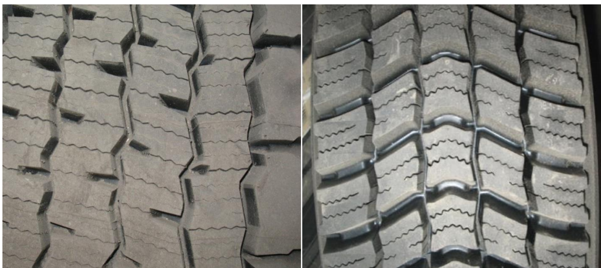
Figure 7. Drive tire tread patterns: wide-base tires (left) and dual tires (right).
