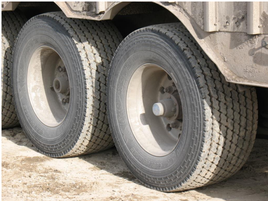
Figure 5. Tires installed for the test stage on the trailer axles of the test truck.
