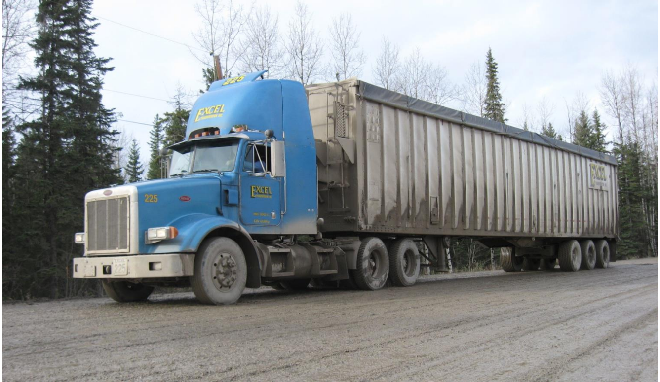
Figure 1. Test truck with wide-base tires on drive and trailer axles.
