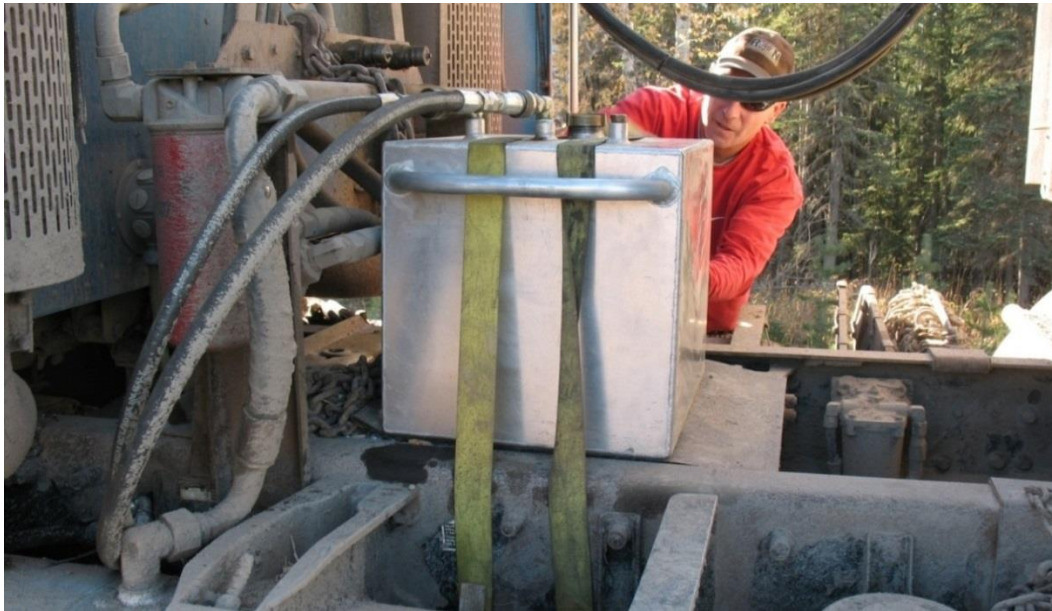
Figure 2. Portable tank installed on a test truck.
