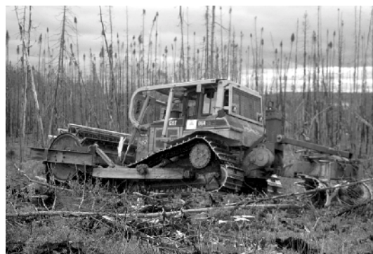
Figure 1. Simultaneous crushing and scarification performed by a bulldozer equipped with a roller-crusher on the front and a passive-disc scarifier pulled behind.
