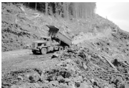
Figure 7. Conventional rigid-frame truck dumping at spoil site.
