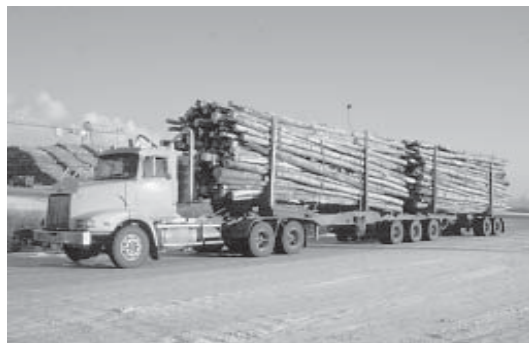
Figure 2. TAC configured B-train equipped with a Redline-Eltek 3-zone TPCS.
