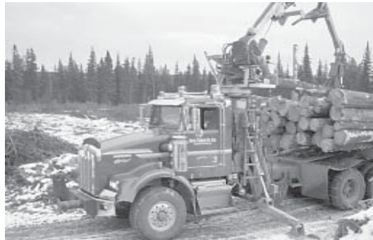
Figure 1. Self-loading 5-axle off-highway truck equipped with an Eaton TPCS.
