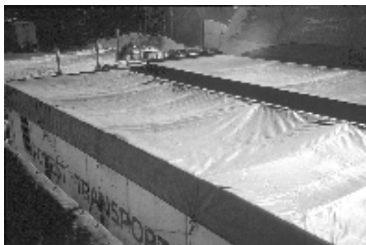
Figure 2. (Left) A tarpaulin in poor condition will contribute to freezing problems. (Right) A well-maintained tarpaulin, properly attached to the trailer, will minimize freezing problems.
