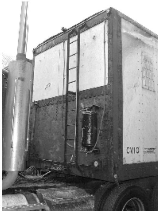
Figure 5. The components of an onboard spray system. (Top) A pressurized tank on the trailer. (Center) The sprayer's spray nozzle. (Bottom) Applying the antifreeze chemical.
