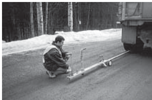
Figure 2. Measuring pavement deflection using Benkelman beam.
