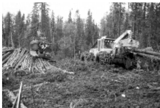
Figure 1. A delimeter and grapple skidder working together in a hot-logging operation.
