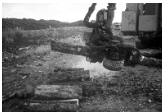
Figure 8. Slashing of stems into 1-m sections with a single-grip harvester to permit an assessment of internal damage.
