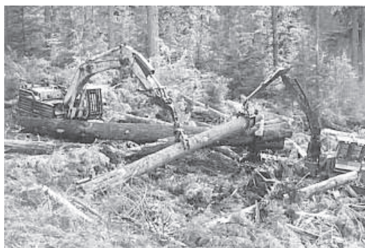
Figure 5. John Deere loader-forwarder assisting clambunk with loading large stems (photo courtesy of Woodima Forestry Services).
