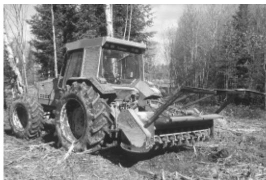
Figure 1. (Left) The Bull Hog BH 150 mulcher mounted on the three-point hitch of a Valmet 8750 tractor.
