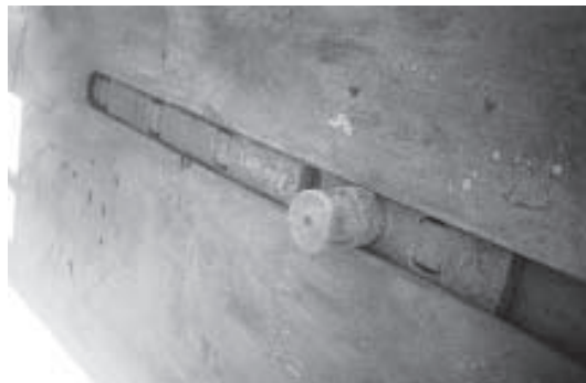
Figure 2. Sliding kingpin mechanism and underside of trailer bolster plate.
