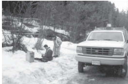
Figure 3. Collecting data from frost and moisture probe data logging station on Philpott Road.
