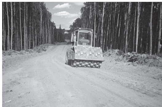
Figure 6. Tamping foot vibratory compactor used on test road.
