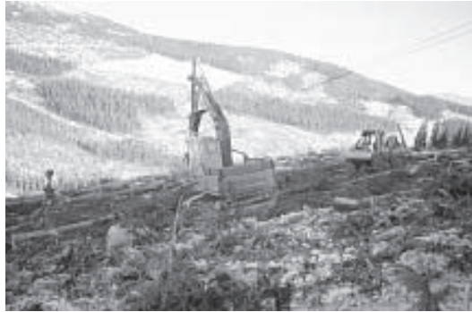
Figure 3. Skidder delivers stems to the loader for transfer to the yarder's grapple. The yarder's grapple grabs stems previously placed in position.
