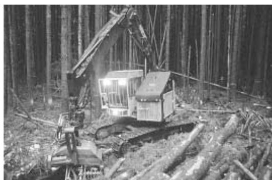
Figure 3. Timbco 415 harvester falling on the SW200 treatment unit.
