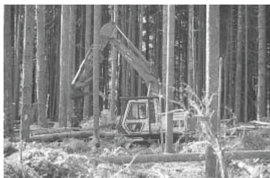
Figure 5. Hydraulic loader pre-bunching logs for yarder.
