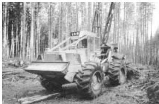
Figure 6. Ranger 667 skidder used to forward and sort yarded logs.
