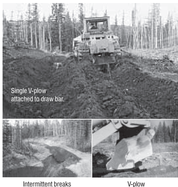
Figure 3. Ripping with moldboard V-plow at Drayton Valley.
