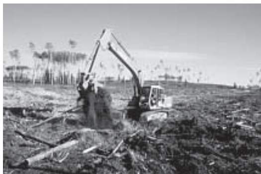
Figure 6. Excavator using site preparation rake during retrieval.
