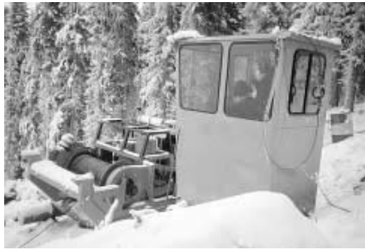
Figure 2. Skylead 6000 Series sled yarder and operator's cab. Strawline drum is not installed.
