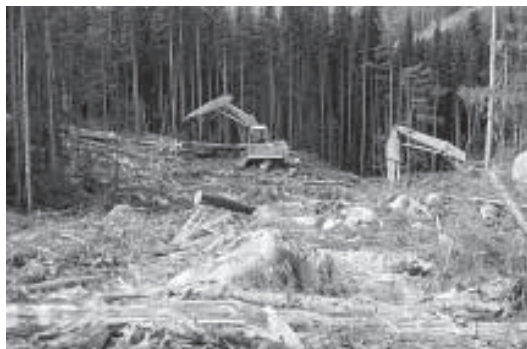
Figure 7. Loader-forwarding in the adverse section of Cutblock 13. Note the surface boulders.
