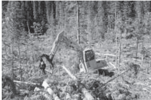
Figure 6. Loader-forwarder working near a riparian management zone to extract stems from between the residual saplings.
