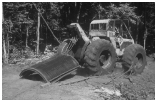
Figure 1. The rugged KWH plastic arch can be easily transported to the installation site.
