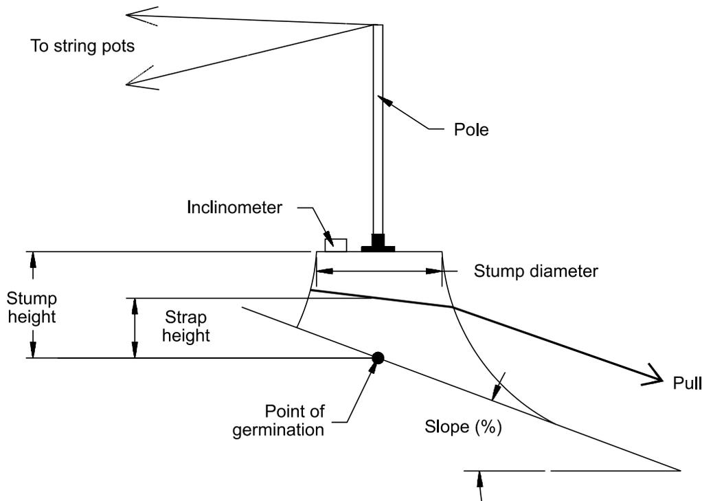
Figure 4. Stump parameters that were measured in the study.
