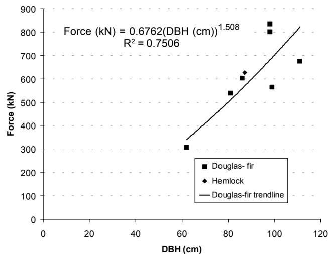
Figure 6. Relationship of ultimate stump strength with estimated DBH.
