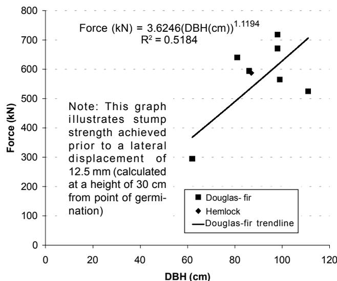
Figure 7. Relationship of stump strength at 12.5 mm lateral displacement with estimated DBH.
