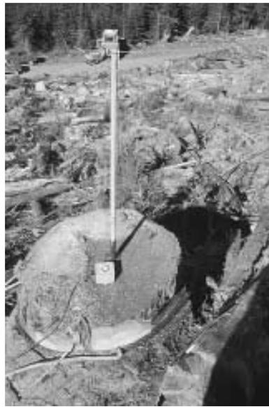
Figure 3. Instrumented stump showing the inclinometer at the base of the pole.
