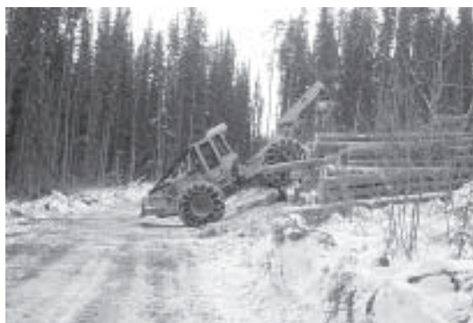
Figure 4. Skidder landing turn at roadside.
