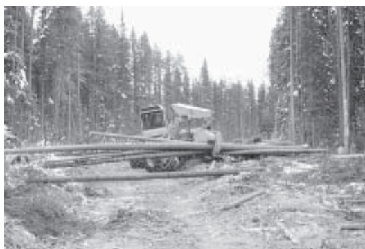
Figure 10. Skidder repositioning stems from a corridor which approached the road at a right angle.
