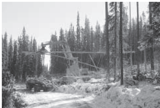
Figure 6. Loader working in patch cut treatment. Residual stand in foreground is vulnerable to stem damage during log loading.
