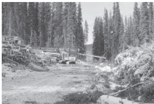
Figure 5. Processor working within the patch cut treatment. An additional cut below the road gave the processor room to feed the full length stems through its cradle.
