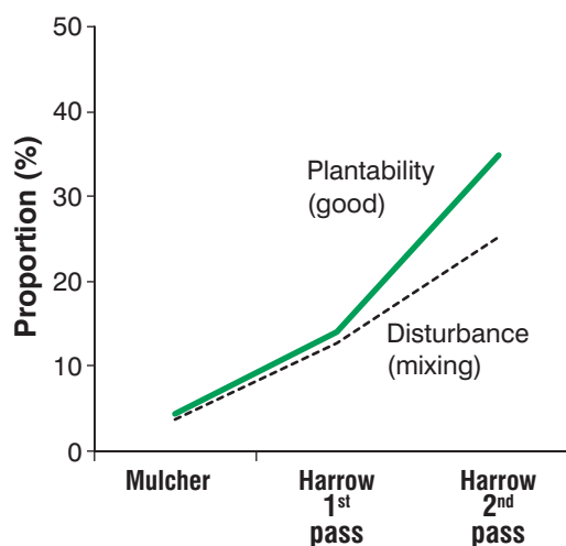
Figure 3. The increase in disturbance after each pass of the machines.
