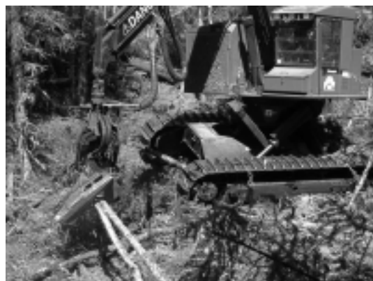
Figure 1. (left) The Waratah HTH-470HD head on a Timberjack 608L carrier in the Charlevoix study.
