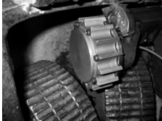
Figure 4. The large measuring wheel used for multi-stem application (photo courtesy of Y. Beaulieu, Waratah Forestry Attachments).
