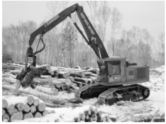
Figure 3. The processing head lets the operator sort the products based on various quality criteria, including the minimum and maximum diameters accepted by each mill.
