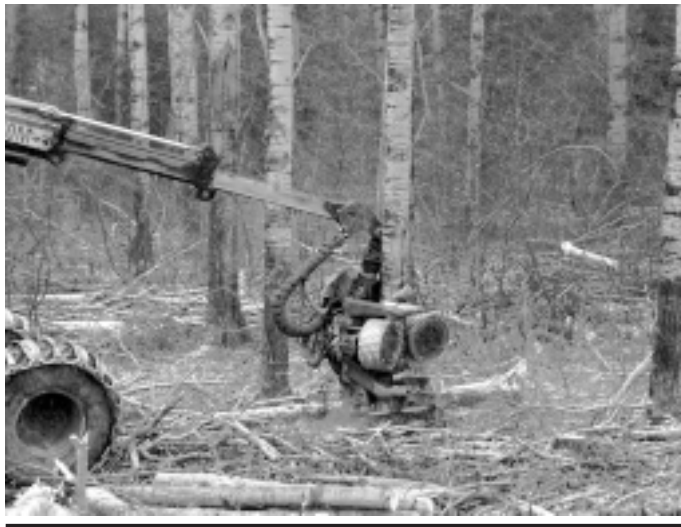
Figure 1. A Valmet 965 single-grip head harvesting aspen.
