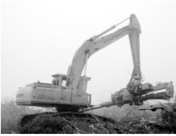
Figure 2. On certain models of processing head, a butt plate helps the operator consistently buck stems at the target lengths.
