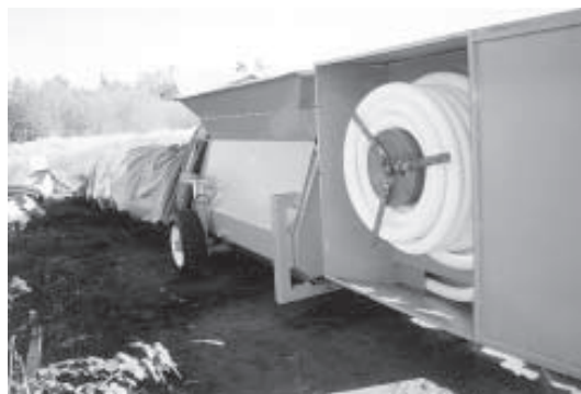
Figure 4. Aeration pipe for the AG-BAG system.
