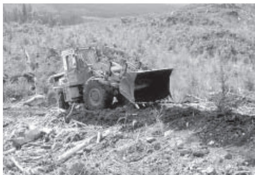
Figure 8. Front-end loader spreading composted material.
