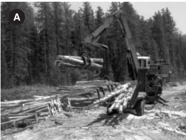
Figure 3. Merchandizing with (A) a roadside slasher and (B) a processor.
