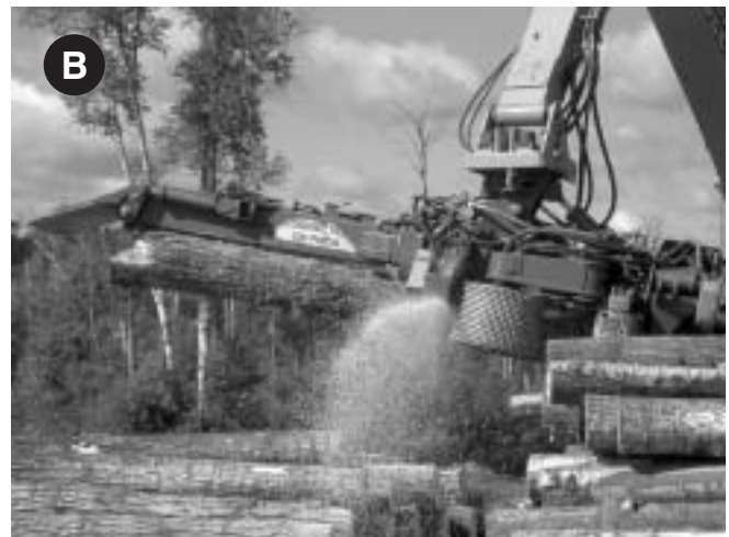
Figure 3. Merchandizing with (A) a roadside slasher and (B) a processor.
