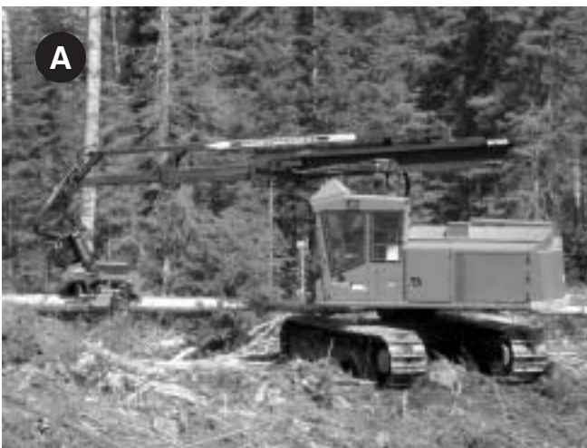
Figure 4. At-the-stump merchandizing using (A) a single-grip harvester and (B) a processor.
