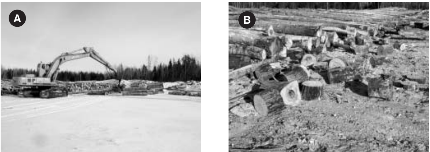
Figure 2. (A) A single-grip processor working in a satellite yard. (B) Rotten sections trimmed from veneer logs.
