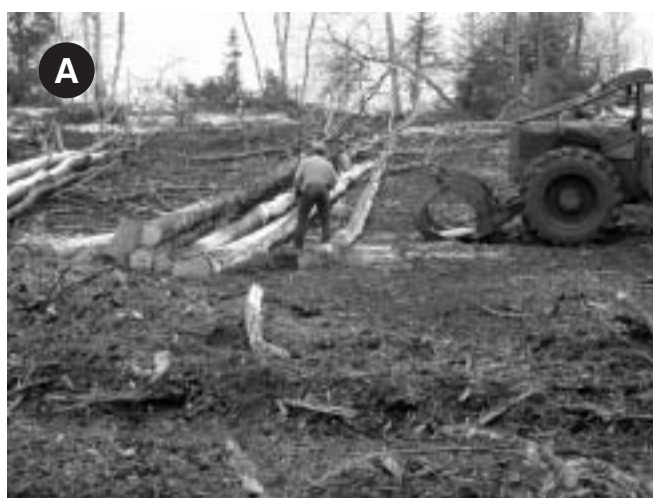
Figure 1. Extraction of veneer logs: (A) Manual bucking and piling with a small cable skidder. (B) Piles after mechanized extraction with a slasher.
