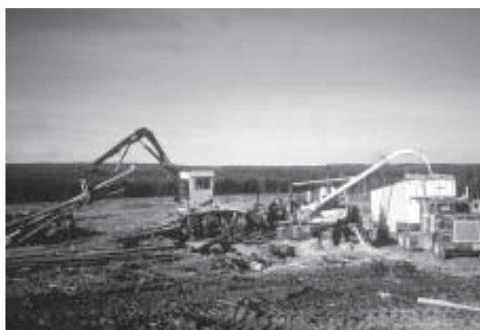
Figure 2. Peterson Pacific DDC 5200 chipping logs near Hinton Alberta.
