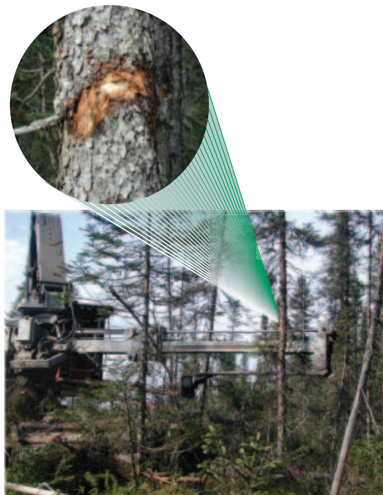
Figure 2. Examples of wounds caused by the processor head (at left) and by the machine's rear overhang (at right).
