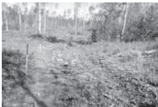
Figure 4. One year after skidding, tilled organic layer on a skidder track subjected to 44 passes.
