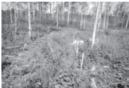
Figure 3. One year after skidding, minimal disturbance of organic layer on a skidder track subjected to 15 passes.
