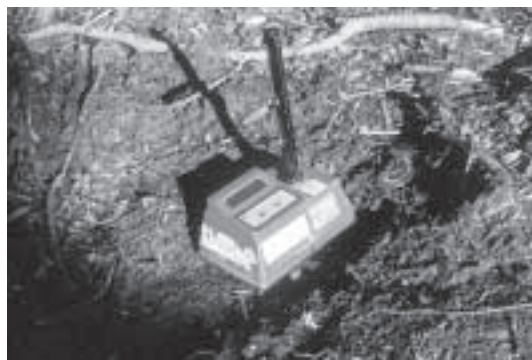
Figure 1. Recording soil bulk density with a single-probe, nuclear, moisture/ density gauge.
