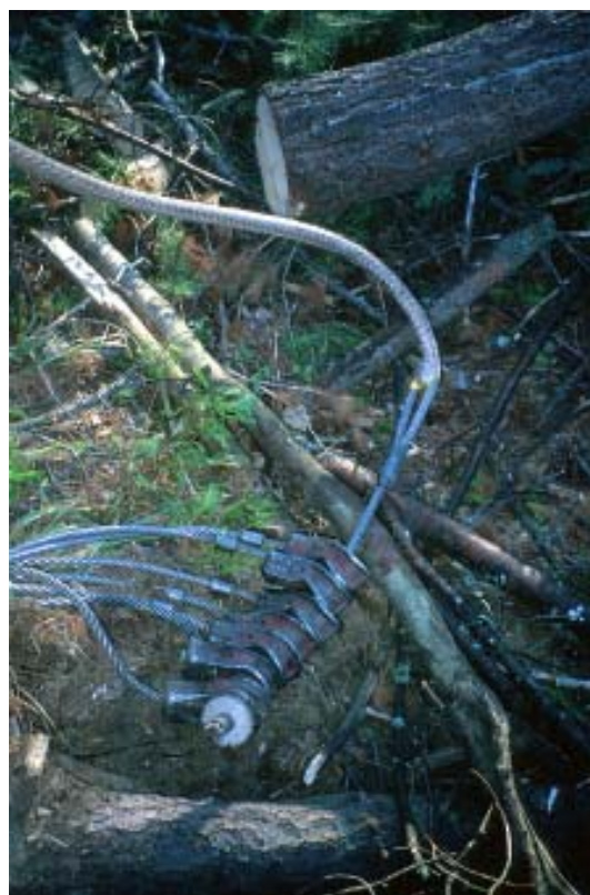
Figure 1. The spliced connection between the Spectra rope and the wire leader.
