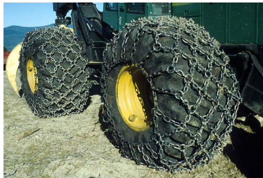
Figure 2. 1.1-m-wide tires and wheel chains.
