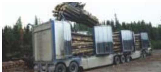
Figure 1. A multi-use B-train designed to haul roundwood and chips.
