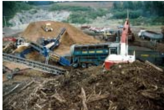
Figure 4. The production of hog fuel from sortyard residues (Forrester 1996).
