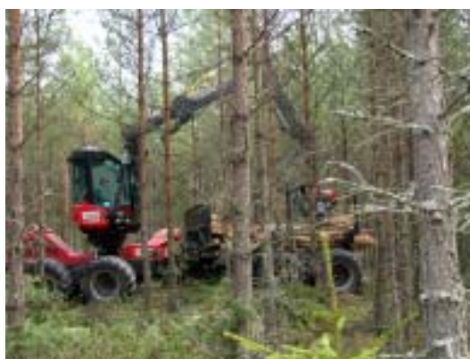
Figure 2. A harwarder (combination harvester and forwarder) has been developed in Scandinavia to fell and forward material to roadside for chipping. In this picture, the harwarder is producing pulp and sawlogs.
