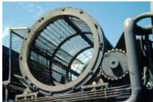
Figure 5. Trommel screen used to classify material entering a water separation unit (Forrester 2000).
