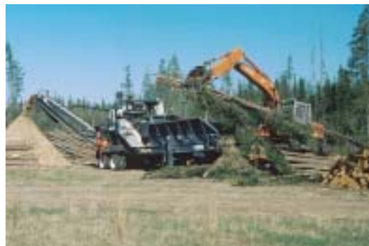
Figure 6. Peterson Pacific 2400 portable hog mill converting harvesting slash to hog fuel in northern Alberta (Forrester 2003).
