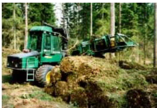
Figure 3. A Timberjack Energy Wood Harvester 1490D biomass baler mounted on a forwarder. One of these units was tested in 2003 by the U.S. Forest Service.
