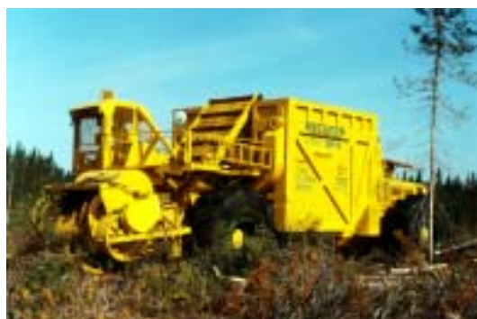
Figure 1. The Recufor was designed to recover logging residue left on the forest floor, to comminute this material, and to transport it to roadside. The high cost of owning and operating the machine compared to the low value of the biomass prevented commercialization of the unit.
