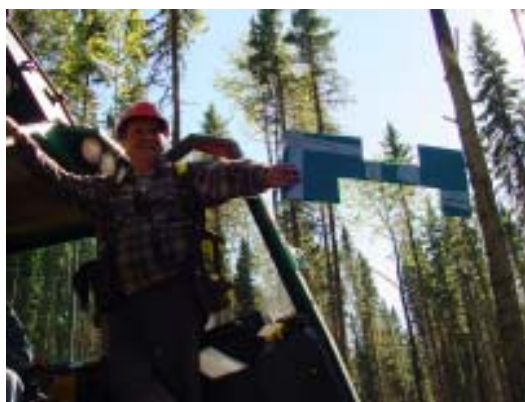
Figure 2. An example of the "cut-no-cut" gauge for the operator.
