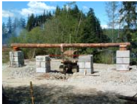
Figure 2. Log stringer in position at test facility.
