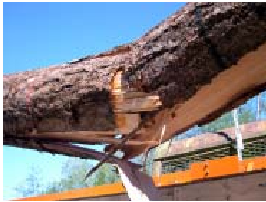
Figure 8. Failed Douglas-fir log in bending test.
