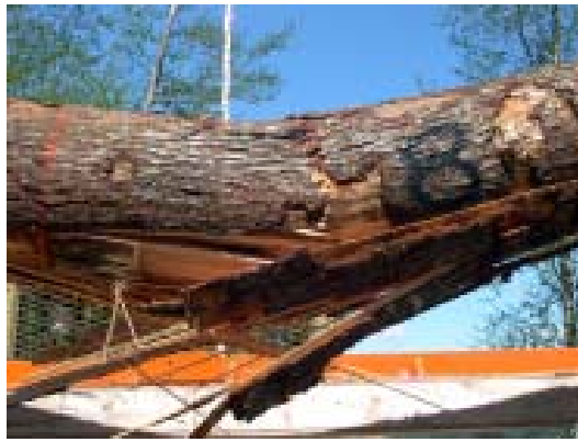
Figure 7. Failed western hemlock log in bending test.
