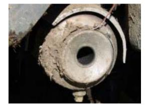
Figure 8. Dried muskeg debris at the end of ATV 1's muffler.
