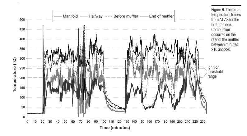
Time for debris to dry. Part of the study was to investigate the length of time required for debris to dry on the exhaust system and thus become susceptible to ignition. By using the data collected by the thermocouples and from observations taken during the ride, the drying process time can be quantified. For example, combustion was observed on ATV 3. Its time-temperature profile is presented in Figure 6.
