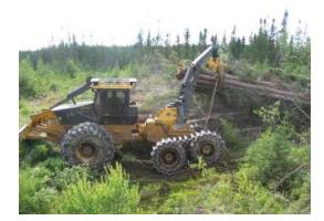
skidder must do. This potentially offers improved protection of advance regeneration. The swing-boom also lets the driver avoid climbing onto the wood piles at roadside, thereby potentially decreasing the stem breakage caused by this practice.
