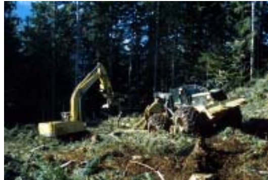
Figure 3. Caterpillar 535B grapple skidder intercepts bunches forwarded by the John Deere 892E LC loader-forwarder.
