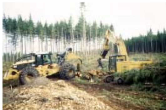
Figure 5. Stems skidded by the Caterpillar 535B are decked by the John Deere 892E LC loader-forwarder.
