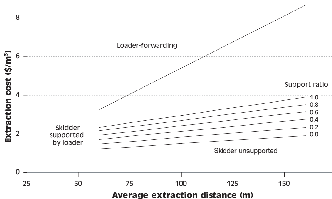
Figure 13. Estimated loader-forwarding and skidding costs as functions of extraction distance and support ratio.
