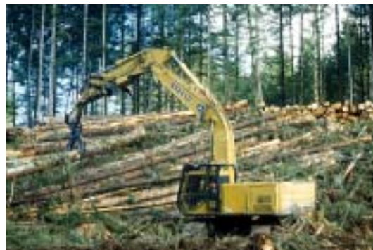
Figure 6. Stems skidded by the Caterpillar 535B are decked by the John Deere 892E LC loader-forwarder below a hillside road.
