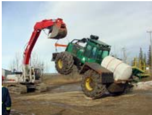
Figure 6. Adverse rollover trial of a Timberjack 460 skidder with a 2270 L tank.
