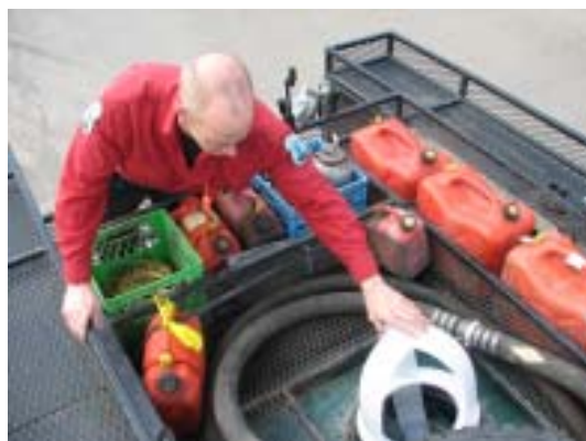
Figure 7. Installation of a Surge Buster® liquid surge control unit (photo supplied by Linbir Holdings Ltd., Kamloops, B.C.).
