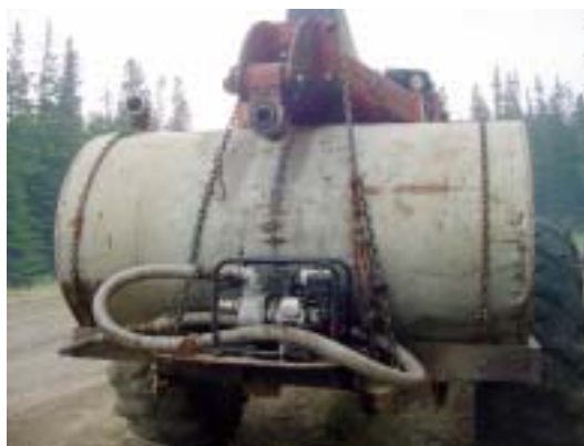
Figure 1. Used oil tank mounted temporarily on skidder arch for water delivery.
