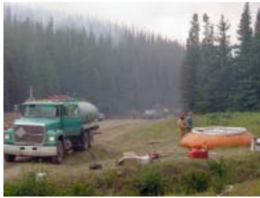
Figure 3. Water truck filling a synthetic portable holding tank (22 700 L) for use by skidder.
