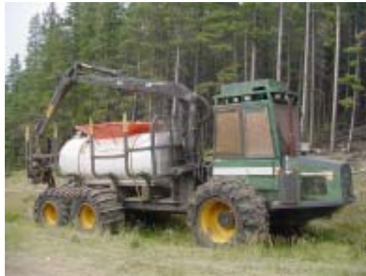
Figure 4. The tank mounted on the FMC forwarder can be filled using a helicopter bucket.
