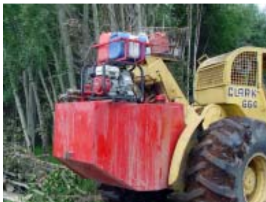
Figure 2. Illustration of a good tank design.
